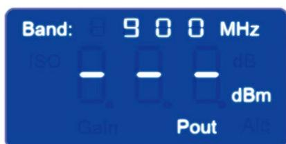
**LCD6:** Displays "-" if the output power is negative,
