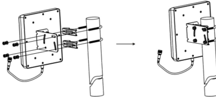
**Note:** Wrap waterproof tape around the connectors between outdoor antenna and feeder line to avoid water or other kind of damage.
