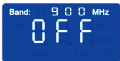
When LCD screen is in "OFF" state and the repeater shuts down, LCD screen will be flashing.
