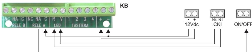
**Example of connection with burglary central units of TM or PROTEC series (excl. PROTEC5X)**
