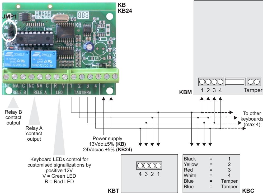
KB24 is a control system with electronic keypad that can drive two relay outputs independently or in combined mode using two customised codes. It can be used to activate and deactivate alarm systems, for access control and for all applications that require a safe and reliable control that is simple to install and to use.
