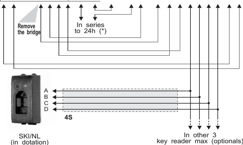
(\*) This connection is optional; if a false electric key is inserted in the connector, the 24h anti-sabotage protection will be active.
