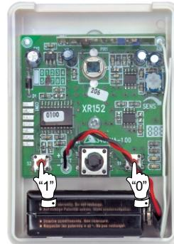
Then enter the 18-digit terminal code, checking that the green LED lights up for one (left button) and the red LED for zero (right button).
